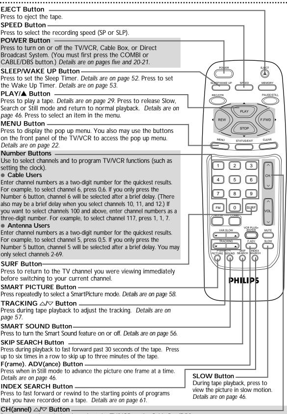
Press to scan through the channels at the TV/VCR or the Cable Box/DBS. When in FM mode, press to select an FM radio channel. *Details are on page 58*.
